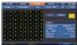
Constellat. DVB-S2 = 8PSK, T & T2 = COFDM, C = QAM and all modulation parameters
