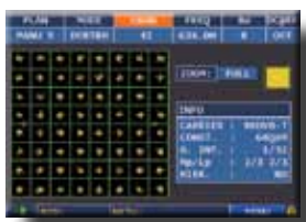
Constellat. DVB-S2 = 8PSK, T = COFDM, C = QAM and all modulation parameters
